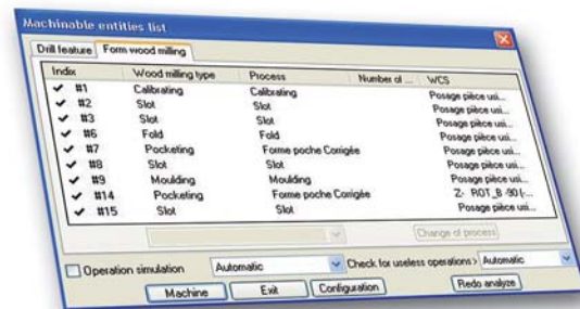
Automatic recognition of geometries for machining operations.
